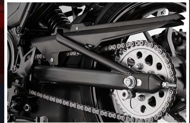
ALUMINIUM SWINGARM IMPROVES CORNERING PRECISION AND RESPONSIVENESS.
