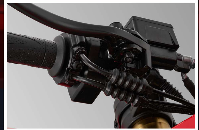
BRAKE CLUTCH ENGAGES OR DISENGAGES ENGINE POWER FOR SMOOTH GEAR SHIFTS.
